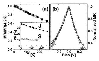
FIG. 4. (a) *T* dependence of the normalized differential MR for sample J ( $\blacksquare$ ) and *S* ( $\square$ ). Inset: same data before normalization; (b) bias dependence of the differential magnetoresistance of sample J (-), and S ( $\square$ ).
