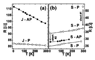
FIG. 1. (a) R(T) for sample J in both the antiparallel ( $\blacksquare$ ) and parallel ( $\square$ ) magnetic states; (b) same for sample S. Open diamond and arrow show *R* before and after the first short was introduced. Small contact, *P* state ( $\square$ ); large contact, AP state ( $\bigcirc$ ); large contact, *P* state ( $\bigcirc$ ).
